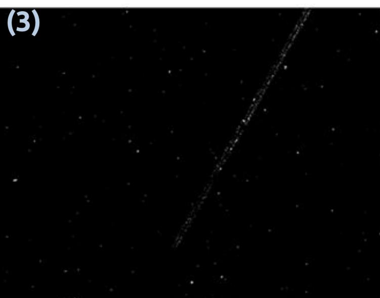
(3) To get a better detection rate image is eroded by a 3x3 erosion kernel. This step removes the noise, but partially destroys linear features as well.
