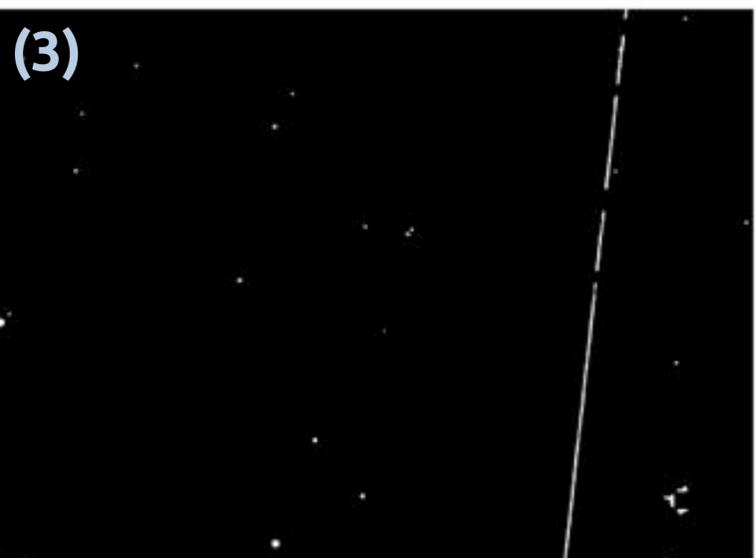
(3) To prepare the image for step (4) image 3 is dilated by 4x4 dilation kernel. This enlarges all existing objects on the image.
