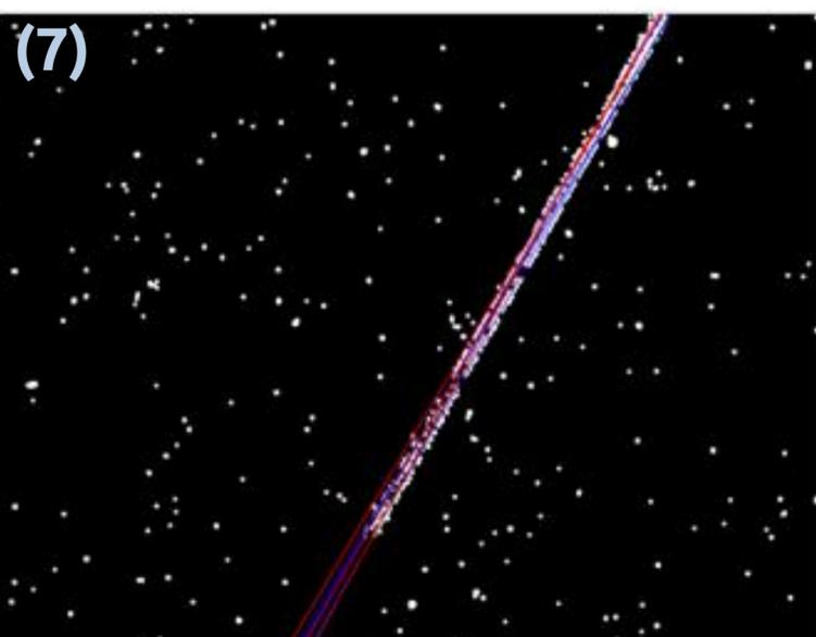
(7) Lines are fitted with Hough line detection algorithm on images 3 (blue) and 5 (red). If those lines have similar coordinates ( $\theta$ ,  $\rho$ ) in Hough space, the detection is True
