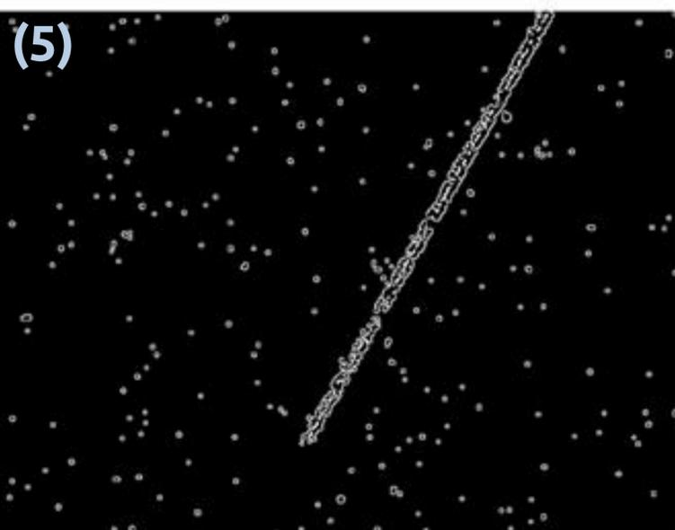
(5) All edges on the image are found with Canny edge detection algorithm.
