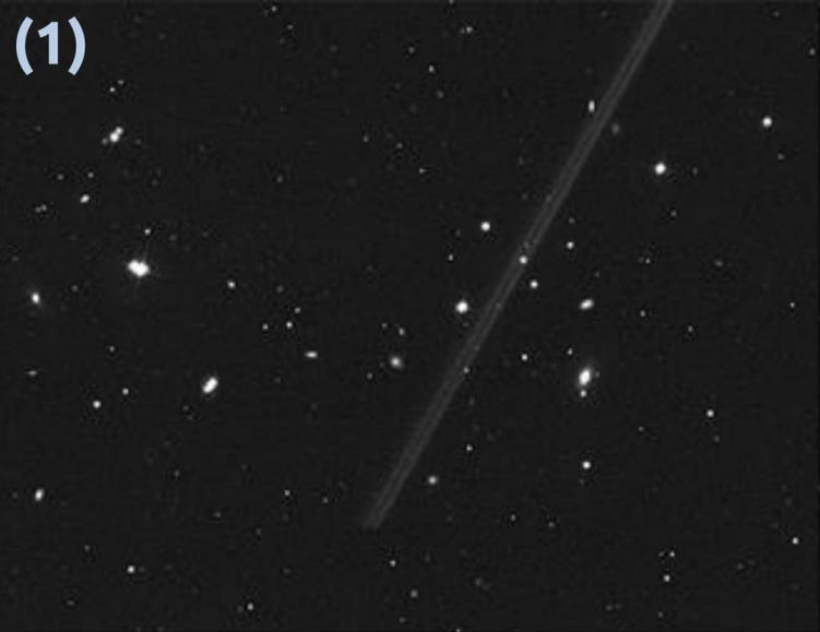
(1) frame-g-002728-2-0424 is an example of a dim trail. Original image 1 is converted from 32 bit float image to 8bit integer image. Pixels with brightness value over 255 are set to 255 and pixels with brightness values less than 0 to 0. Known objects are removed from the image.
