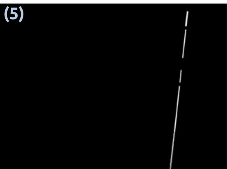
(5) Among the edges only closed looped are kept. Minimal area rectangles are fitted over such contours. Only those rectangles for which longer to shorter side length ratio is larger than  $lwTresh$  are used for image reconstruction.
